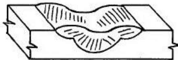
(B) DOWNHILL WELD (1/8 SLOPE)
