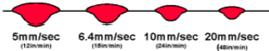
Effect of Arc Travel speed (All other parameters unchanged)
